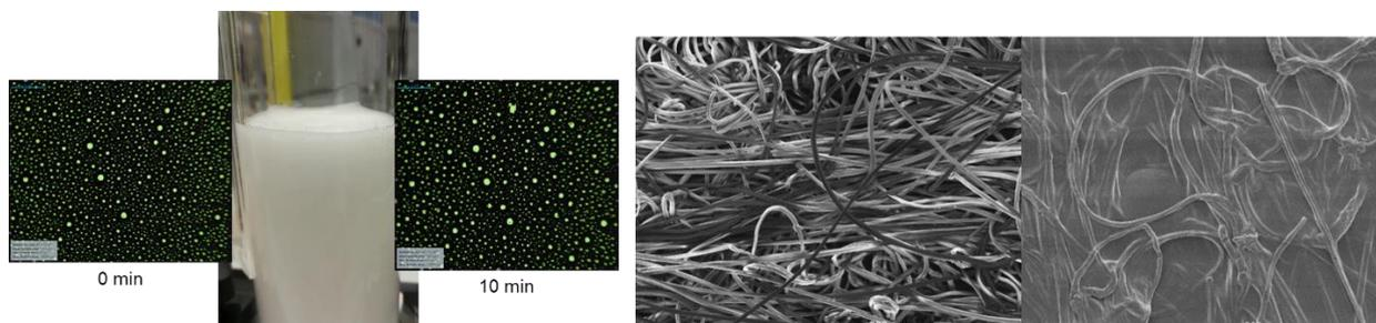
Figure 3. Foam characterisation with the Dynamic Foam Analyzer Krüss DFA100 (left). The SEM pictures of viscous fabric without and with 10 g/m<sup>2</sup> TEMPO-CNF coating layer applied with the foam coating in laboratory scale (middle, right).
