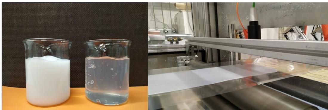
Figure 5. Used industrial MFC or TEMPO-CNF materials (left). On line measurement based on optical confocal technique for measuring film thickness of cast coated layers on plastic in pilot scale.
