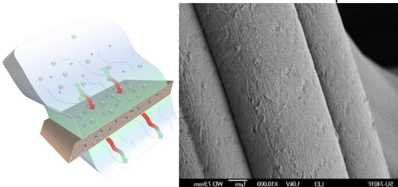
Figure 2. A barrier layer that allows some molecules, ions or small particles to pass through the membrane while some others are stopped (principle of filtering with a membrane or filter, left). Cast coating nanocellulose creates nanotextured surface on cellulose non-woven fabrics (right, the SEM picture of the nanotextured surface).
