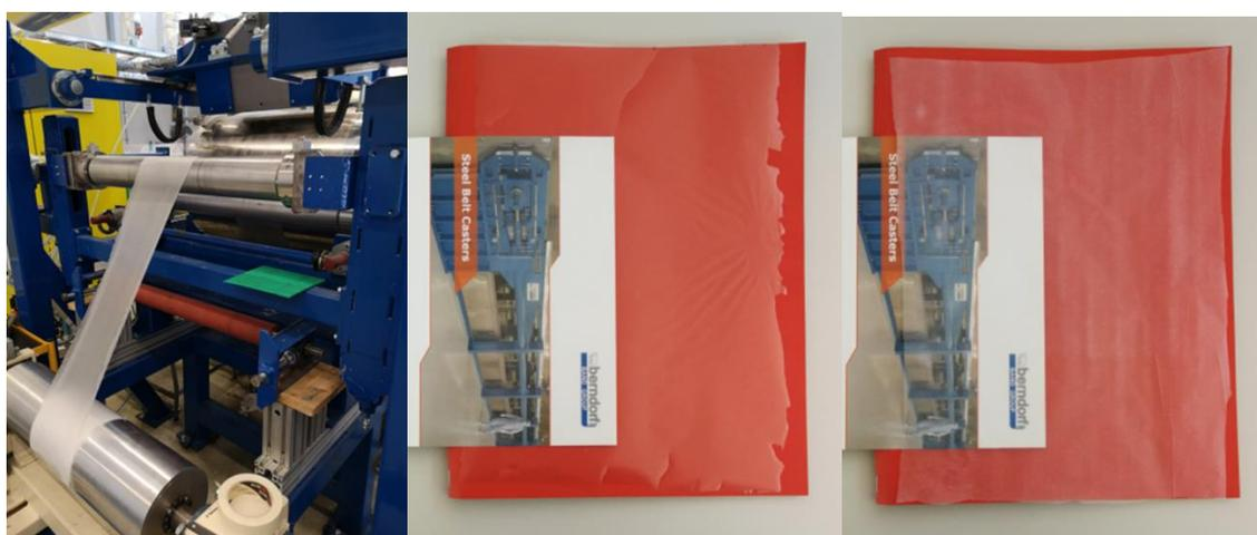
Figure 4. Pull off and winding of nanocellulose film in dynamic conditions (left). Casted Films from nanocelluloses (middle, transparent film from TEMPO-CNF and right, translucent film from industrial MFC).
